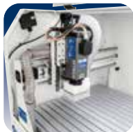
2,4 kW Electrospindle unique in its category
